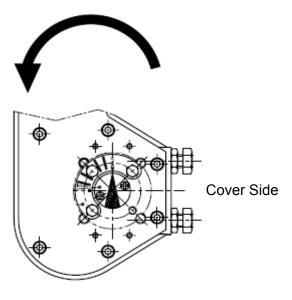
Counter - Clockwise Rotation Clockwise on Fail
