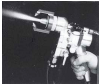
ultra-sonic spray coating for ball and seat
